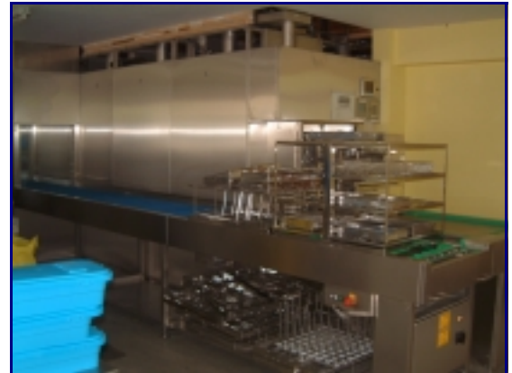
New sectional washer/ disinfectors. Capable of cleaning up to 45 surgical sets per hour
